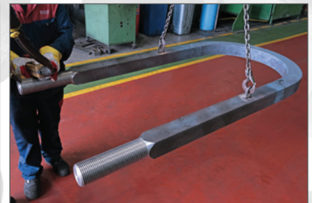
Each M80 U-Bolt measures 782mm wide and 1600mm tall overall.
