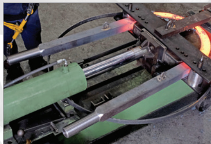
We successfully bent the U-bolts to an inner radius of 311mm.
