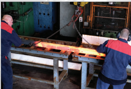
A furnace was constructed to isolate heating at the center point.
