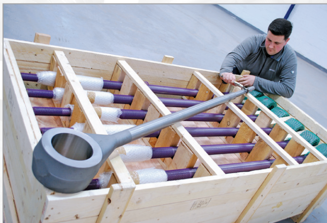
We designed wooden shipping cases to keep the components safe during transport.
