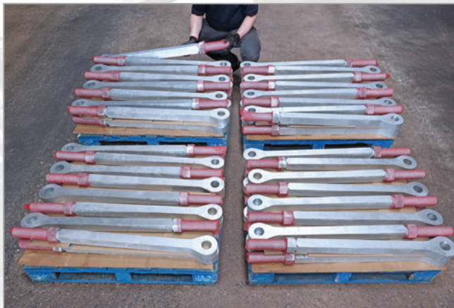
A total of 86 'square' type hanger rods, 2.25" BSW, were supplied to the restoration project.
