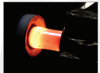
Electrical resistance heating of the bar end.
