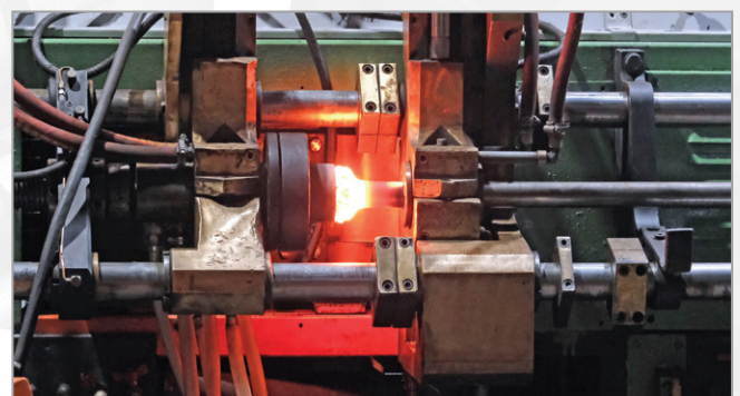
Electrical resistance heating and hydraulic pressure is used to gather material from a single heat.
