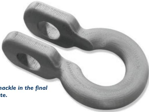
*3D Printed Shackle in the final machined state.*
